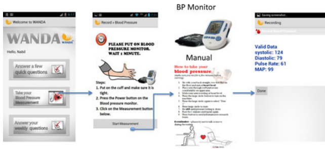
Fig. 3. Snapshot of the WANDA-CVD application showing the steps necessary for the patient to measure their BP. They simply take their BP measurement, then push a button on the application to transfer the data to the phone, which is then uploaded to the server. The participants can also see their data on the phone to validate that the data was received.
