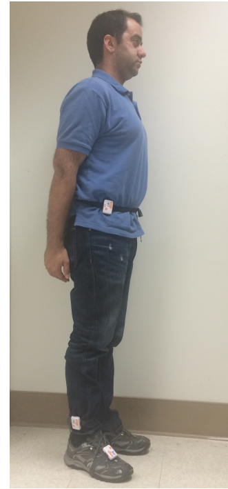
Fig. 1. User wearing sensors on the hip, ankle, and foot for collection trial
