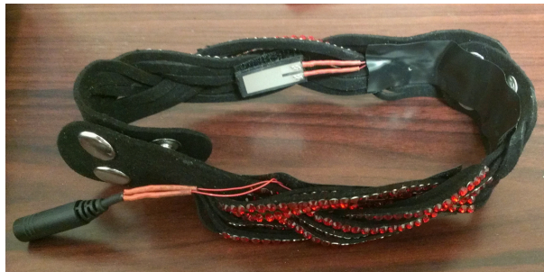
Fig. 2. This figure shows one variant of the necklace including the embedded piezoelectric sensor used to detect swallows
